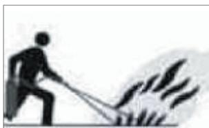
3. Extinguish by squeezing the lever a number of times. Do not empty the extinguisher all at one time.
