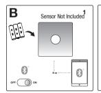
Purchase the Nordlux Sensor. Put the battery into Sensor. Turn on the Bluetooth of your phone. Stay within 8 meters from the Sensor
