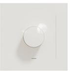
Product description:SmartDim universal rotary dimmer for dimming LED, ohmic, inductive or<br/>capacitive loads. The dimmer is 1-pole.<br/>Use of neutral wire is optional.<br/>Minimum load 0W with neutral, 7W without neutral.<br/>Maximum load to 200W.<br/>Improved dimming performance.It can also be controlled by using impulse switches to control the light from
